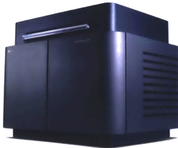
Figure 2: A Stratasys Objet500 Connex. Stratasys produces the Connex series, the only multi-material 3D printers currently on the market. Image from the Stratasys website [7].
