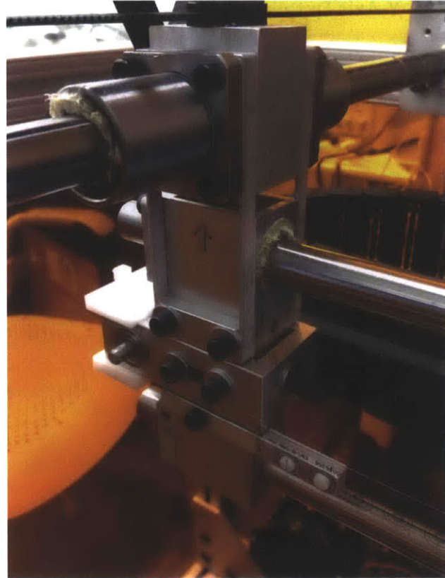
Figure 13: A CAD model of one end of the X-axis (left), showing the flexures (highlighted in yellow), and a photo of the flexures on the actual printer (right). The flexures were cut from aluminum sheet on the waterjet and allow the Y-axis bearings to shift laterally to compensate for misalignment and thermal expansion, while still supporting the weight of the X-axis.
