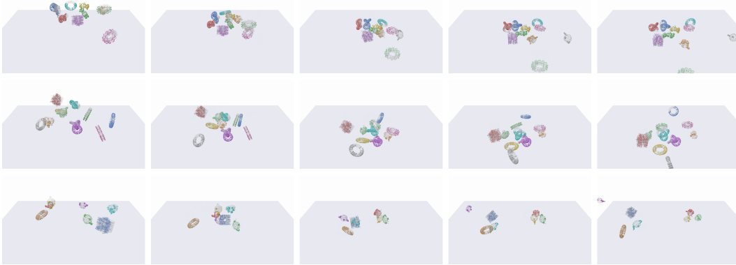
Figure 4: Partial point-cloud rollouts. Three example sequences (rows) where 25% of each object’s points are masked at test time. RigidFormer produces stable rollouts with accurate inter-object contacts. Meshes are shown only for visualization; our model operates on point inputs.
