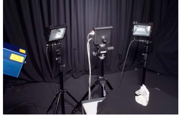
Figure 8.8: Acquisition setup. The laser projector illuminates the target object (resting on the turntable). The scene is observed by the HDR video camera from several positions. The two spotlights visible on both sides of the camera in the right image are used to illuminate the object during silhouette detection.
