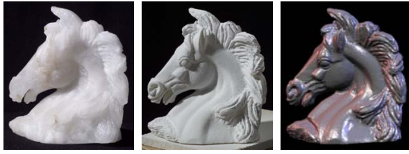
Figure 5.2: The alabaster horse. Left and middle: Photographs of the sculpture with and without subsurface scattering under identical illumination conditions. The sculpture was covered with fine dust to “turn off” subsurface scattering. Much surface detail is masked by the translucency and active optical range scanning systems have grave problems to scan the translucent object. Right: Rendering of the acquired geometry model (100 k triangles) with flat shading.
