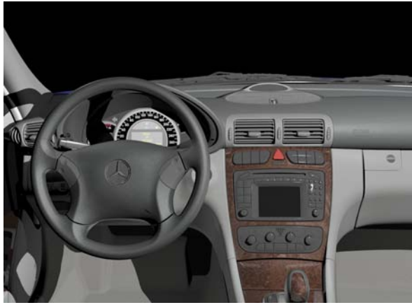
Figure 11.10: Visualization of car interior (Mercedes C-class) with point light illumination. The leather and wood materials are modeled by BTFs. All other materials are standard phong.
