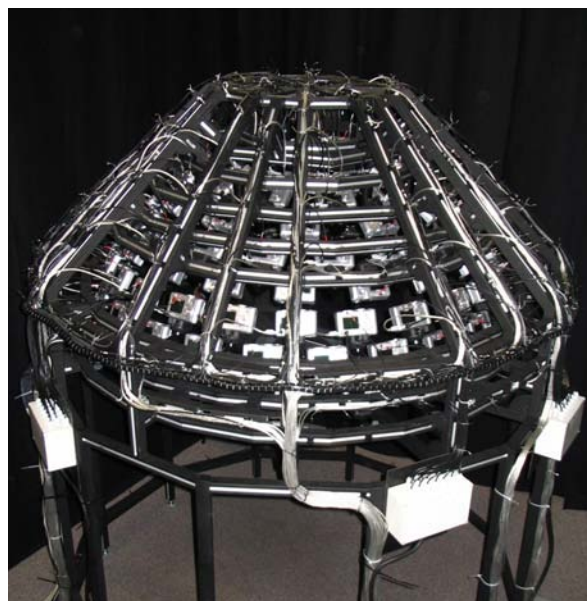
Figure 11.5: 151 digital cameras with built-in flash lights are mounted on a gantry, focusing on the sample, which is placed in the center of the hemisphere.
