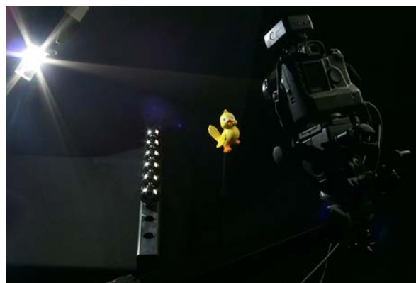
Figure 7.3: Picture of the acquisition setup in a photo studio covered with dark felt (from left to right): point light source, metal spheres for light source tracking, object to be measured, digital still camera.
