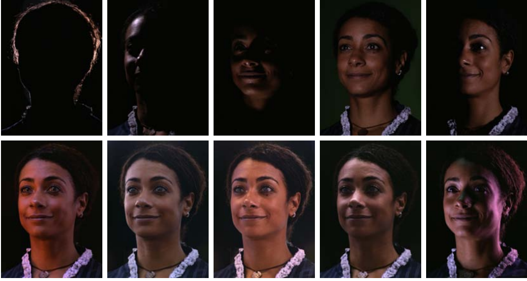
Figure 12.3: The top row shows several captured basis images of a subject under different directions of illumination. The bottom row shows image based relightings of a subject under different environmental illumination.
