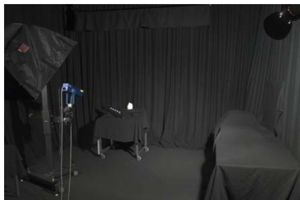
Figure 5.10: The acquisition lab at the MPI Informatik. A test object on the table is illuminated by two HMI light sources with different reflectors.
