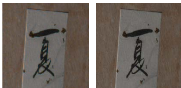
Figure 5.4: Left: Interpolation artifacts in an image acquired with a Bayer pattern sensor (Jenoptik ProgRes C14, single shot, fast reconstruction). Right: Ground truth image acquired using 4-shot mode (see Section 5.2.4 for more details). Note also the visually higher resolution of the ground truth image.
