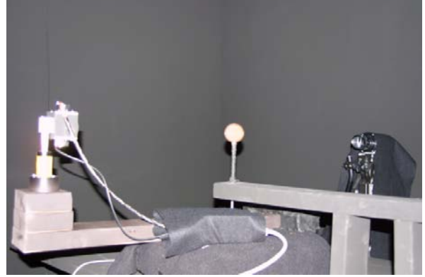
Figure 6.2: A photograph of our high-speed BRDF measurement gantry.
