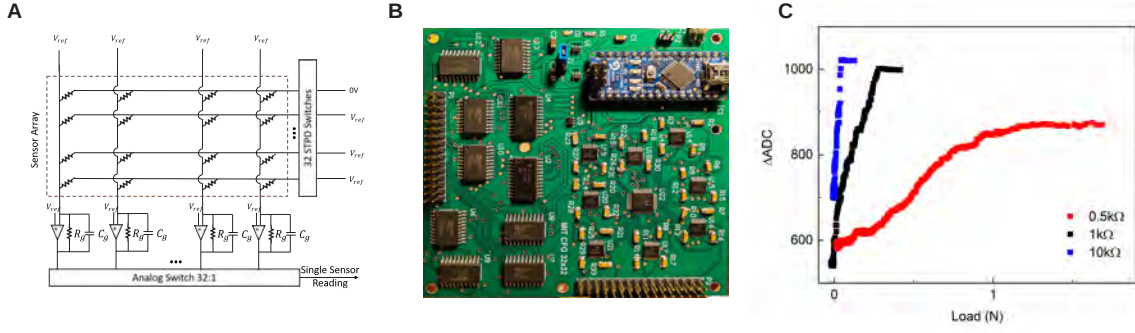
Figure 3-6: A. A modified electrical-grounding-based isolation circuit architecture for passive sensing array readout. B. the designed PCB board. C. The response of a single sensor in response to applied load at the output of ADC.
