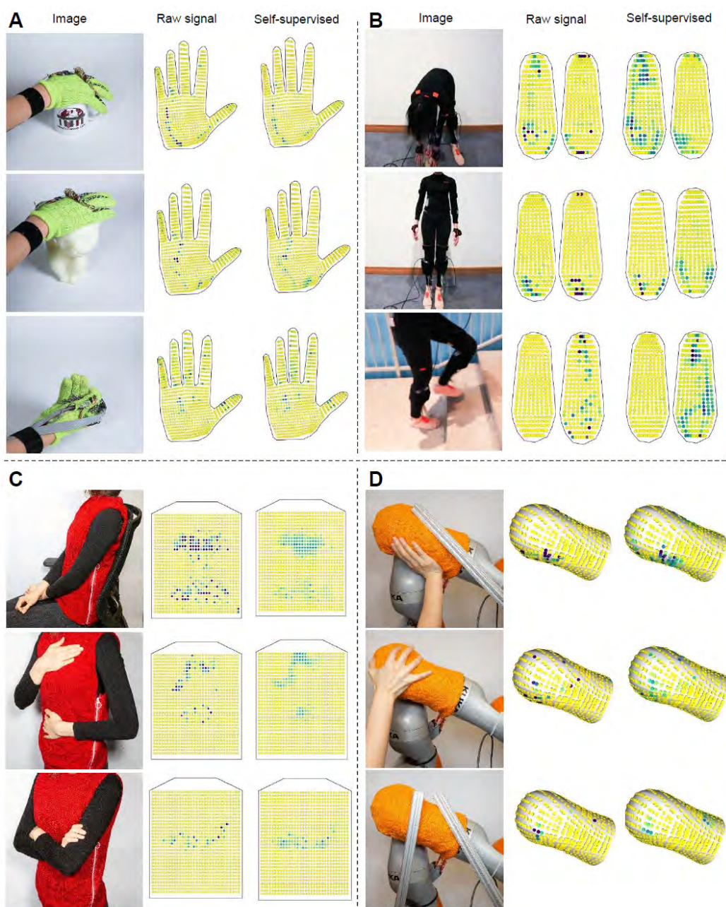
Figure B-1: Examples of self-supervised corrected results of tactile A. glove, B. sock, C. vest, and D. robotic arm sleeve.
