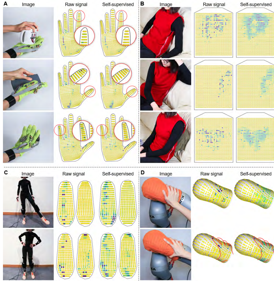
Figure 4-8: Self-supervised correction results on the tactile A. glove, B. vest, C. sock, and D. robot arm sleeve.
