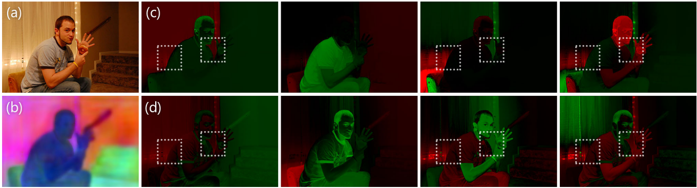
Fig. 5. The image (a) and semantic features (b) are shown with several eigenvectors corresponding to the smallest eigenvalues 1 of the proposed Laplacian matrix (c, top row) and the matting Laplacian as used in spectral matting [Levin et al. 2008b] (d, bottom row). Green represents the positive values of an eigenvector while red shows negative. Our Laplacian matrix strongly reveals the semantic cuts in the eigenvectors while the matting Laplacian eigenvectors extend beyond the semantic edges, as the highlighted areas show.
