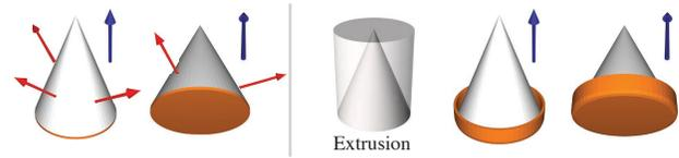
**Figure 11:** A failure case in leaving one free direction for shell computation (left). In this case the up direction was specified, but the shell computation process stops before achieving the stopping criteria, while leaving more than one free direction. The process stops because no triangle can be added without blocking the up motion. A solution to this can be found by expanding the holder on an extrusion of the object along the free motion direction (right).
