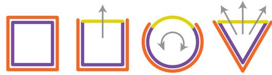
**Figure 9:** Concept of intrinsic free motions. These 2D schematic examples show areas for holder expansion (purple), constrained regions (yellow), “maximum” holders (orange), and intrinsic free motions (gray).
