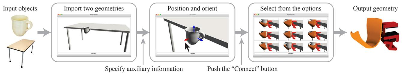
**Figure 2:** User experience. *AutoConnect* requires a simple input to obtain a functional connector. Our method generates many connectors and allows users to choose the best one. Users can also specify some auxiliary parameters such as a free motion direction and a region on the object that should not be covered.
