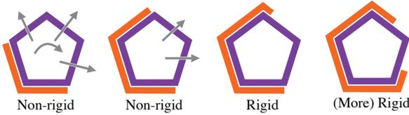
**Figure 8:** 2D schematic examples of our rigid and non-rigid cases. If there is no free-motion, we consider it is rigid; otherwise, it is non-rigid. Purple and orange parts correspond to the target and holder meshes respectively. Gray arrows correspond to free-motions.
