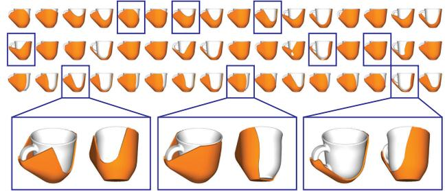
**Figure 12:** (Top) 48 mug holder candidates are generated, from which the 9 holders annotated with boxes are selected by the clustering-based selection algorithm. (Bottom) Close up views of some selected mug holders.
