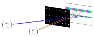
**Figure 10:** A naive automultiscopic display, composed of a pinhole array and a screen where each viewer row sees different pixel rows on the screen. To enable coherent content, one needs to use different horizontal scaling on the angular images intended for viewers in different rows. Thus, resolution tradeoffs here are worse compared to our design.
