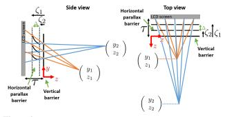
**Figure 4:** Display principle: For each viewer  $(y_i, z_i)$  (orange and blue), there exists  $\zeta_i$  such that a barrier placed at that screen distance leads to proper disparities for viewers at distance  $z_i$ . Concatenating all row-dependent barrier positions  $\zeta_i$ ,  $i = \{1, ..., m\}$  provides the desired shape of the slanted horizontal parallax barrier.
