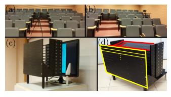
**Figure 16:** Our prototype and capture setup. (a) The auditorium in which images were captured. A camera was placed on a rod and was moved horizontally to simulate the movement of a viewer's head. (b) Capturing was performed at several seats in the auditorium. (c) The barriers assembly and the LCD screen behind it. (d) Emphasizing the vertical barrier (yellow) and the horizontal slanted barrier (red).
