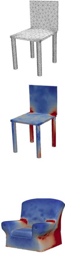
Fig. 49. **Finite Element Analysis for Chair Mechanics.** GPT-4 determines if the chair will break by performing FEM-based stress analysis. In images, the top chair analyzed is designed by GPT-4 in Figure 9 with von Mises stress displayed from blue (zero) to a maximal value (red). A second chair with mesh from an external source is analyzed using the same code.
