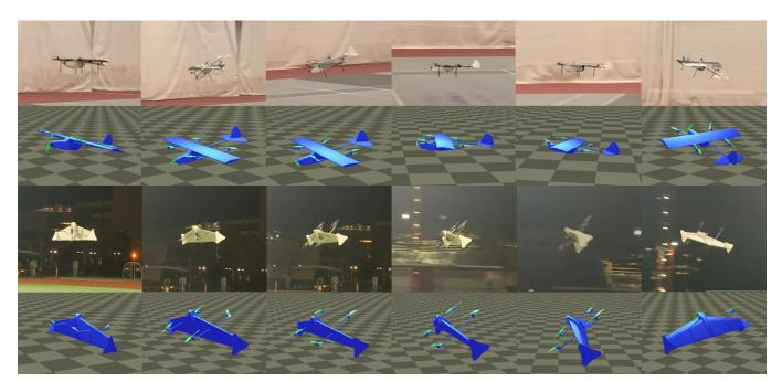
Fig. 8. The quad-plane (model 1) and the tail-sitter (model 2) are transitioning from loitering to gliding (row 1 and 3). Their corresponding flight simulation are shown below (row 2 and 4).
