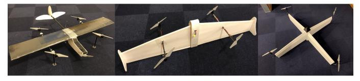
Fig. 6. The fabricated hybrid UAV models. From left to right: quad-plane (model 1), tail-sitter (model 2), x-wing (model 3).
