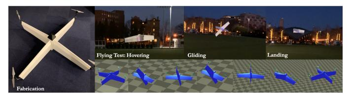
Fig. 1. We propose a computational approach to automatically design a mode-free, model-agnostic neural network controller for customized hybrid UAVs (left). Our novel reinforcement learning framework enables the training of a controller in a stochastically enhanced physics simulator (right bottom) and the crossing of the gap between simulation and reality (right top).
