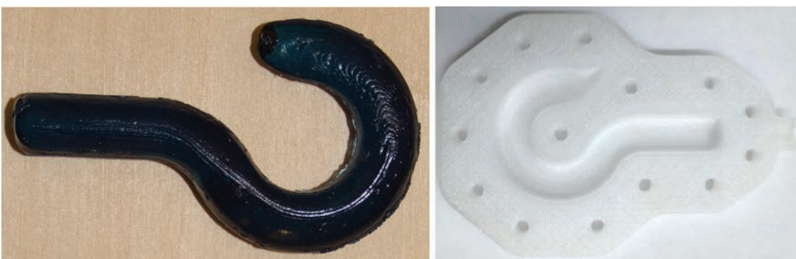
Figure 7. A mechanical hook colored with cyan pigment. The mold (right) is printed with an FDM printer using a clear filament.
