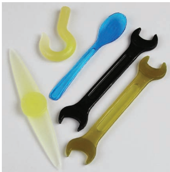
Figure 2. Example objects fabricated with FabSquare. From left to right, clockwise, we can see a propeller with phosphorescent pigments, a hook with silica particles, a spoon with colored pigment, a carbon fiber wrench with an embedded RFID tag, and a second wrench mechanically reinforced with clay particles.
